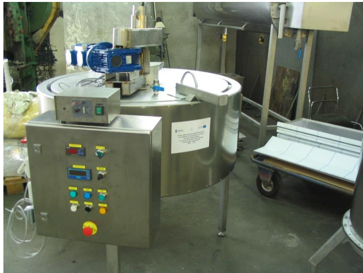
Fig. 2 Reactor for biomass digestion with innovation mixing system
